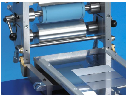
Detail of K Printing Proofer Flexo Head
